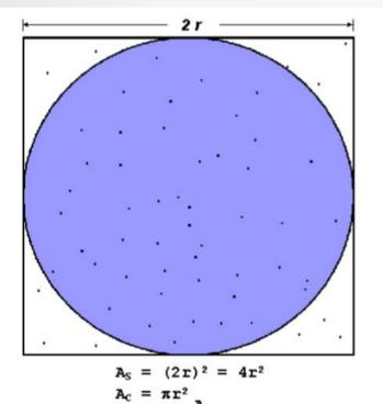
If a program picks N points (x, y) at random inside the square. If a point is inside the circle (i.e. if  $x^2 + y^2 < R^2$ ) M is incremented by one.
